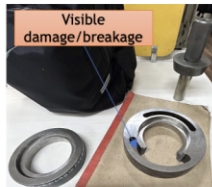
Visible damage/breakage Modified dolly (0502AAA08150F014)
